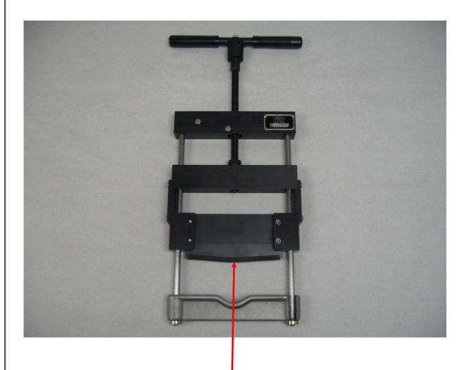
Raise blade while wearing gloves. Remove rubber guard before cutting pipe
