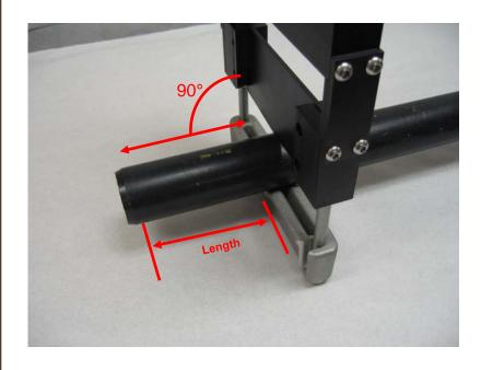
Minimum suggested cut length is pipe diameter
