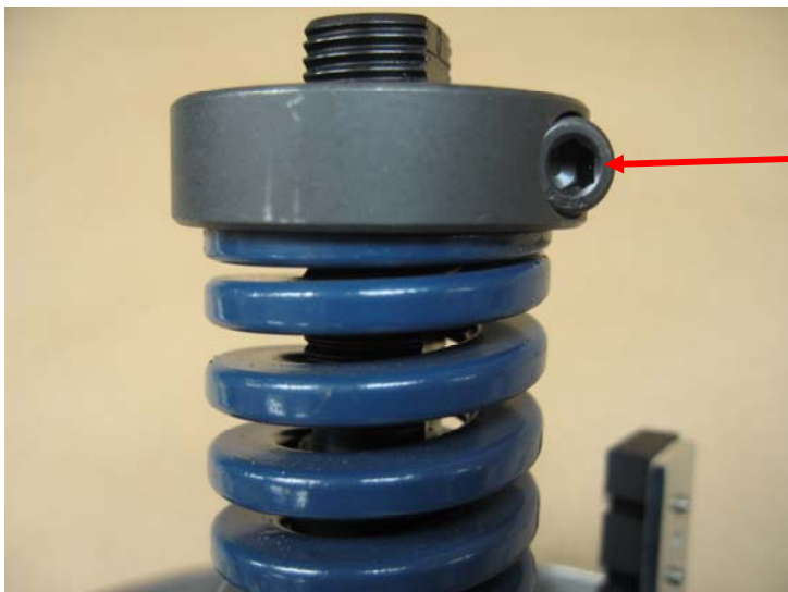
Turn the collar to increase the torque
