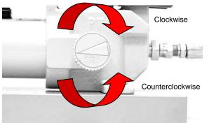
9. Turn valve clockwise on the pump until it is HAND TIGHT. DO NOT USE A WRENCH. Make strokes necessary to snap pipe. Turn knob counterclockwise to release valve after cut to retract piston.
