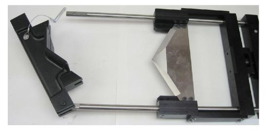
Turn handle and open blade all the way. Pull pin to allow bottom of V-Base to swing out. Place cutter over pipe. Swing V-Base back and replace pin.
