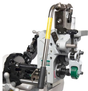
9700 Hydraulic Roll Groover on Threader.
