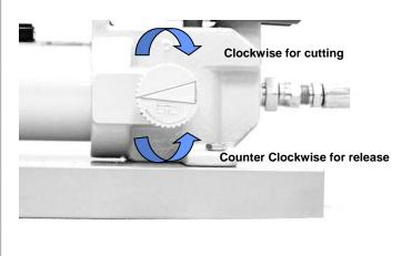
8. Turn valve clockwise on the pump until it is HAND TIGHT. DO NOT USE A WRENCH. Make strokes necessary to snap pipe. Release valve after cut to retract piston.
