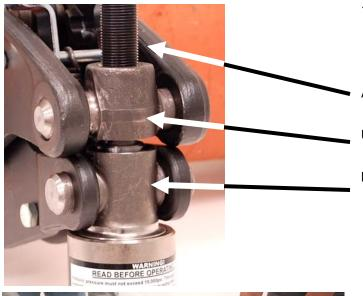
1. Turn adjusting screw until outer collar is at it's <u>lowest</u> limit of travel. Do this for <u>EACH</u> cut.
