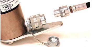
8. Attach hydraulic pump to cylinder. Remove dust cover from coupling, insert hydraulic hose end and turn threaded coupling sleeve until tight by hand.
