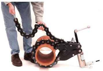
Using hand ring, pull chain over pipe and under tie bolt, then up between jaws as tightly as possible.
