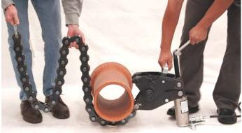
2. Slide chain under pipe at location of cut.
