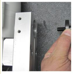
Install #275118 SHCS and #701014 Washer into the counter bored hole of #700996 Lower block. This will secure the block to the drill body
