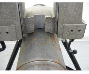
Make sure the machined "V" in the bottom of the frame is centered on the pipe.
