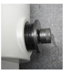
Using an Allen Key, tighten the Plug into drill body.
