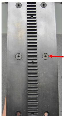
Install (4) #276888 ¼-20 Flat Head Cap Screws into Plate. Tighten all (4) screws using an allen key.
