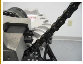
Pull the chain upward and place into the Chain Hook Block #700993. (see below)
