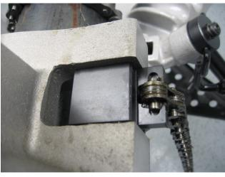
Once chain is hooked into the block, turn Handle #606742 in the clockwise direction to tighten frame to pipe.
