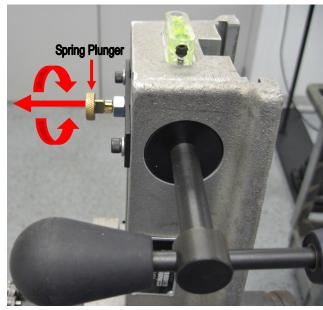
Pull Retractable Spring Plunger #276899 out and turn 90 degrees. This allows the feed handle to turn freely.
