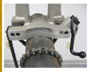
Both the #700993 Chain Hook, and the #700985 Chain Tension Block can be relocated to the opposite sides of the #700975 Frame if needed to fit in tight quarters.
