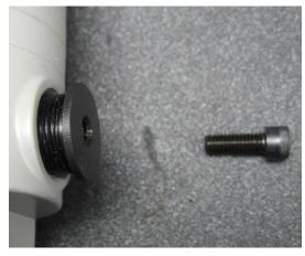
Remove #275118 Socket Head Cap Screw from #701015 Plug.
