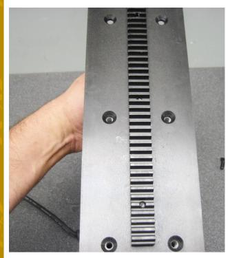
There are (6) holes located on the #701063 Plate. These holes are equally spaced to mount in a few different configurations to the #700996 Lower Block. This allows the operator to change for drill stroke requirements or overall space requirements.
