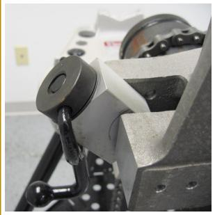
Turn Handle counter clockwise to lower Chain Screw threads.
