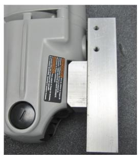
Install the following parts (#700996 Lower block, #701190 Key, #701111 Adapter Block-Milwaukee, (2) #275016 Socket Head Cap Screws) over #701015 Plug as shown.
