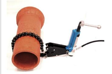
2. Slide chain under pipe at location of cut.
