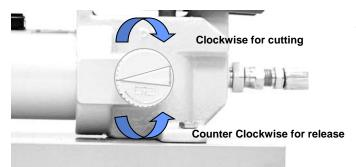
8. Turn valve clockwise on the pump until it is HAND TIGHT. DO NOT USE A WRENCH. Make strokes necessary to snap pipe. Turn knob counterclockwise after cut to release valve and retract piston.
