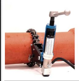
Pull chain over pipe and under tie bolt, then up between jaws as tightly as possible. Allow chain to relax so nearest pin is engaged in slots under upper nose jaw. Chain then can be folded over on itself.
