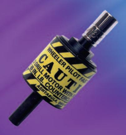
Tighten or loosen No-Hub couplings in just seconds with the Wheeler-Rex No-Hub coupling wrenches. Designed for use with virtually any 3/8" reversible, electric drill, No-Hub coupling wrenches are easily chucked or un-chucked as any drill bit. These unique No-Hub wrenches feature an automatic clutch within the torque head to prevent over or under tightening. Recalibration can easily be done with a torque wrench.
