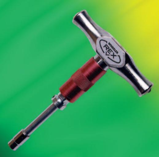
"T-Handle" type torque wrench features a unique locking collar, which enables the wrench to be used as an untorqued snug-up or back-off tool or as a conventional torque wrench. Retracting the locking collar allows the tool to torque right (tightening), while ratcheting to the left. When proper torque value has been attained, an internal slip mechanism eliminates the ability to over-tighten.
