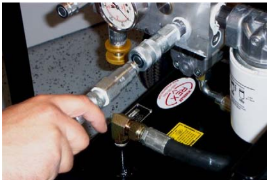
Lines being attached to the Power Pack
